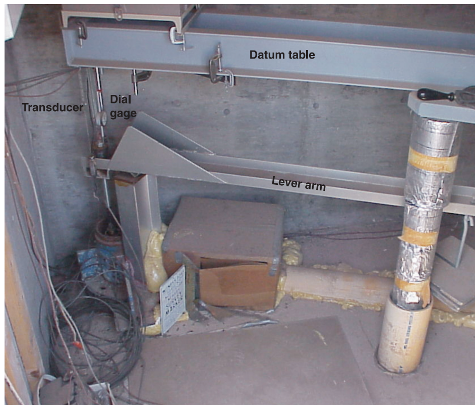
Figure 3. Photograph of shallow extensometer lever arm, datum table, and selected associated instruments.
