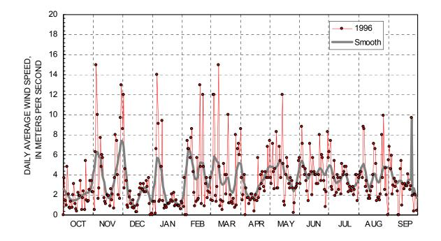
Figure 8. Daily average wind speed recorded at 1,480-meter weather station in Gulkana Glacier Basin, 1996 hydrologic year. Smooth is an inverse distance weighted smooth of the data using an 11-day window.
