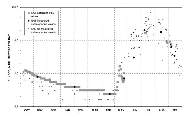
Figure 15. Estimated daily runoff from Phelan Creek near Paxson, 1996 hydrologic year (USGS stream-gaging station 15478040), with measured values for both 1996 hydrologic year and entire period of record (1967–78, 1990–96).
