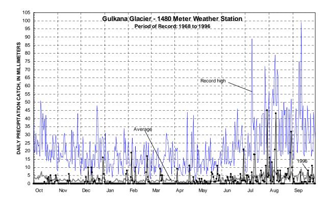
Figure 7. Daily precipitation catch recorded at 1,480-meter weather station, Gulkana Glacier Basin, 1996 hydrologic year. Also shown are record high and average daily precipitation catch since 1968.
