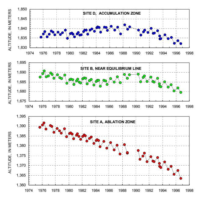
Figure 12. Glacier-surface altitudes at index sites A, B, and D. An unresolved datum shift exists between the 1975–87 data and the 1988–96 data.
