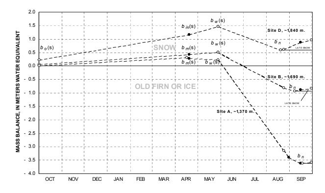
Figure 4. Time distribution of index-site mass balances for Gulkana Glacier, 1996 hydrologic year. Solid circles are measured values; open circles are estimated values. Seasonal maximum balances occurred during late May.  $b_0(s)$ , initial snow balance at site;  $b_m(s)$ , measured winter snow balance at site;  $b_m$ , net balance at site;  $b_w(s)$ , maximum winter snow balance at site. Site altitudes are approximate long-term averages rounded to the nearest 10 meters.
