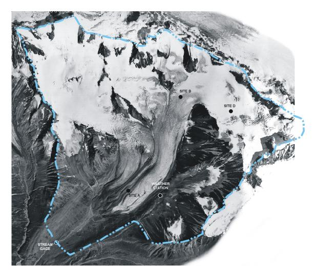
Figure 3. Composite vertical photograph of Gulkana Glacier and its basin showing index-measurement sites, streamgaging station, weather station, and basin boundary, July 11, 1993 (photographs Gulkana GI 1 No. 5 and Gulkana GI 2 No. 4 by AeroMap U.S., Inc.). A, B, and D are measurement sites for mass balance, ice motion, and surface altitude. Dash-dot-dot-dash line indicates basin boundary.
