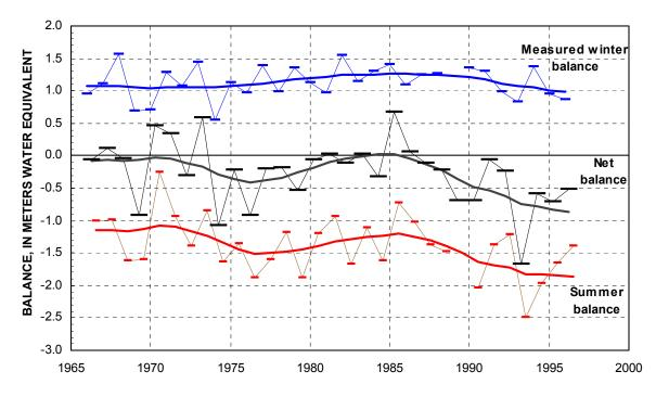
Figure 11. Glacier-averaged measured winter balance, net balance, and summer balance, 1966–96, and smoothed data. Horizontal length of data symbols represents approximate time period of each data value. Smooth is an inverse distanceweighted smooth of the data using a 7-day window.
