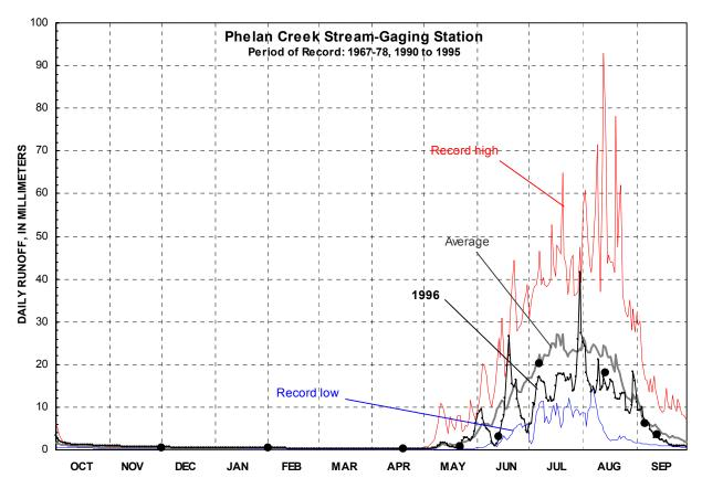
Figure 14. Daily runoff from Phelan Creek near Paxson (USGS stream-gaging station 15478040), 1996 hydrologic year. Large filled circles are instantaneous discharge measurements, expressed as runoff, that are used to define the stage-discharge relation. Also shown are the record-high, average, and record-low daily runoff for the period of record (1967–78, 1990–96).
