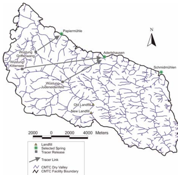
Figure 7. Hydraulic connections established through dye tracing.
