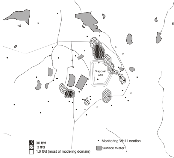
Figure 2. Hydraulic conductivity distribution of upper model layer, based on aquifer testing.
