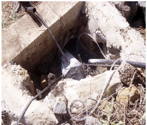
Figure 3. Plankton nets were used to collect club moss spores from the west and east hatchery springs. Spores were used as surrogate tracers (33 microns) for the whirling disease parasite.
