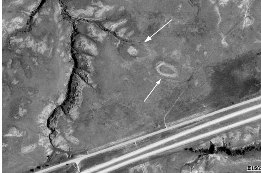
Figure 31. Aerial photograph of two sinkholes (arrows), about 500 feet long, aligned along head of gully suggesting that the present drainage controls the location of the sinkholes. These are 3,700 feet northeast of the Buffalo Jump.
