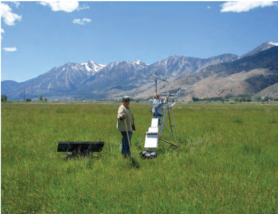
D. Three-dimensional eddy-correlation station at site ET-4 in stand of flood-irrigated pasture. Depth to the water table is from 3 to 4 feet below land surface. Looking southwestward towards the Carson Range.
