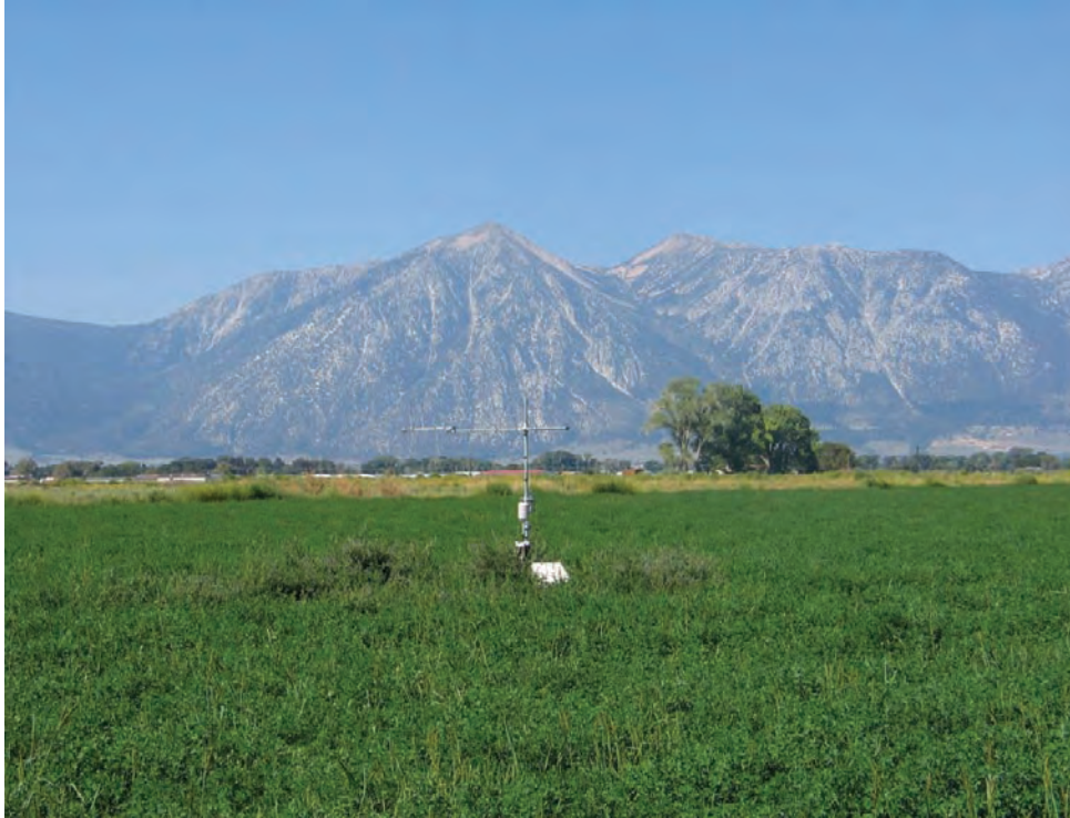
E. One-dimensional eddy-correlation station at site ET-5 in stand of flood-irrigated alfalfa. Depth to the water table is about 40 feet below land surface. Looking westward towards the Carson Range.
