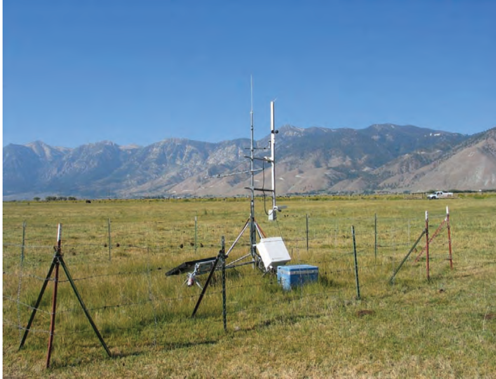
C. Bowen-ratio station at site ET-3 in stand of flood-irrigated pasture. Depth to the water table is from 2 to 5 feet below land surface. Looking southwestward towards the Carson Range.
