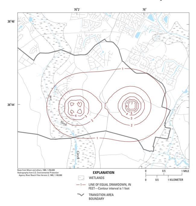
**Figure 15.** Simulated drawdowns in the sand aquifer of the Yorktown confining unit (model layer 4) caused by pumping 150,000 gallons per day at a golf course (maximum drawdown of 5 feet) and 150,000 gallons per day at a hypothetical neighborhood (maximum drawdown of 7 feet) in the Transition Area of Virginia Beach, Va.
