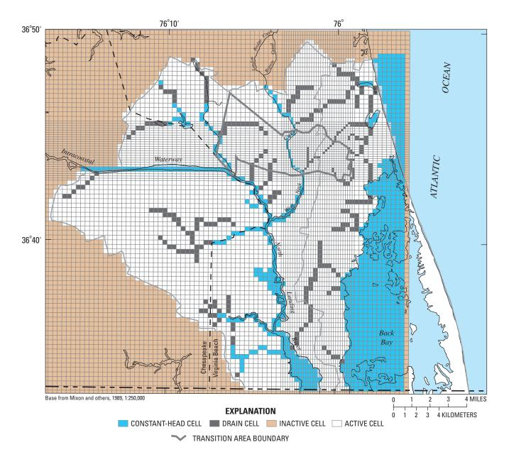
Figure 6. Refined grid and boundaries of the ground-water flow model of the southern watersheds of Virginia Beach, Va.
