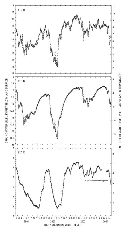
**Figure 4.** Water-level measurements from the spring of 2001 to the spring of 2004 from continuous recorders in the shallow aquifer system in Virginia Beach, Va. (See figure 1 for well locations.)
