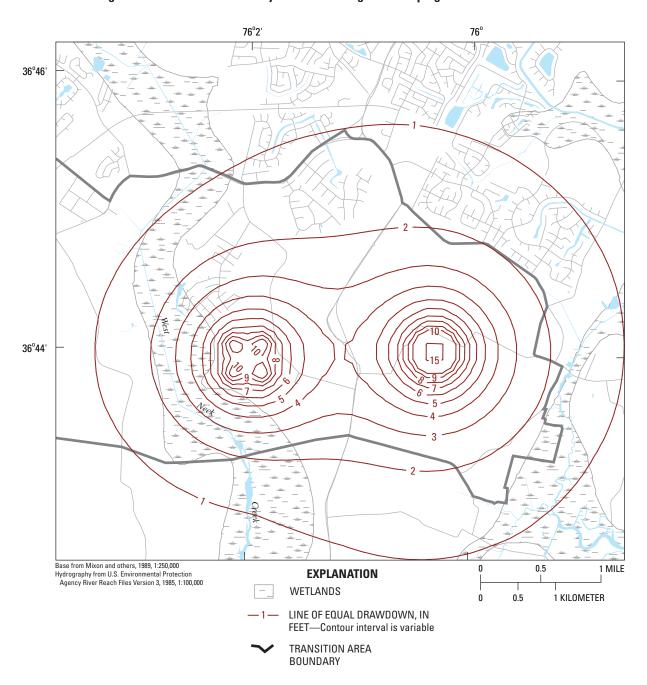
**Figure 14.** Simulated drawdowns in the sand aquifer of the Yorktown confining unit (model layer 4) caused by pumping 300,000 gallons per day at a golf course (maximum drawdown of 10 feet) and 300,000 gallons per day at a hypothetical neighborhood (maximum drawdown of 15 feet) in the Transition Area of Virginia Beach, Va.
