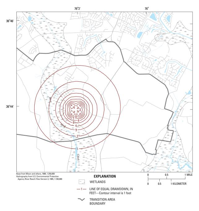
**Figure 10.** Simulated drawdowns in the sand aquifer of the Yorktown confining unit (model layer 4) caused by pumping 300,000 gallons per day at a golf course in the Transition Area of Virginia Beach, Va.
