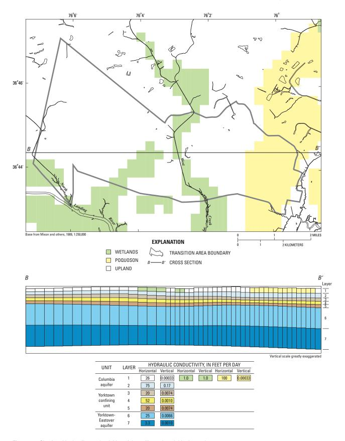
Figure 5. Simulated hydraulic conductivities of the calibrated model in the study area.
