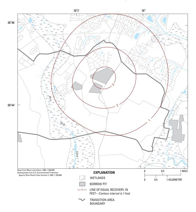
**Figure 9.** Simulated recoveries in the sand aquifer of the Yorktown confining unit (model layer 4) caused by cessation of dewatering at two borrow pits in the Transition Area of Virginia Beach, Va.
