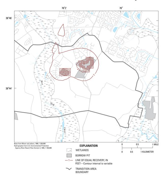
**Figure 8.** Simulated recoveries caused by cessation of dewatering at two borrow pits in the Transition Area of Virginia Beach, Va.
