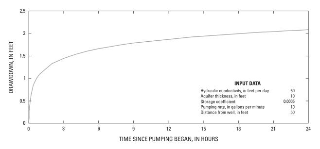
**Figure 11.** Drawdown 50 feet from a well pumping 10 gallons per minute from the sand aquifer of the Yorktown confining unit, according to the Theis (1935) non-equilibrium equation.
