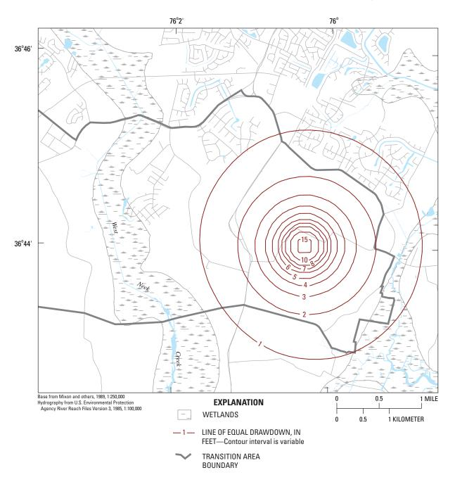
**Figure 13.** Simulated drawdowns in the sand aquifer of the Yorktown confining unit (model layer 4) caused by pumping 300,000 gallons per day at a hypothetical neighborhood in the Transition Area of Virginia Beach, Va.
