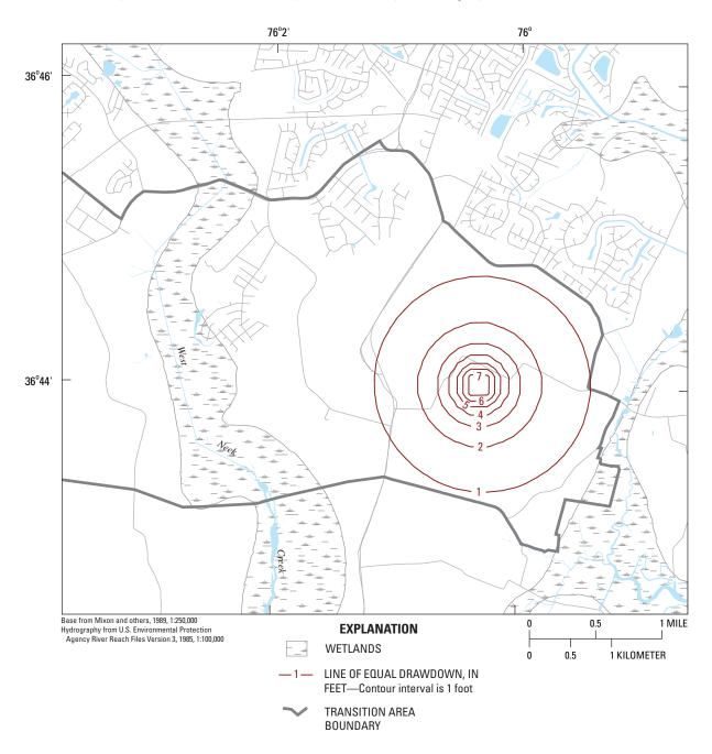
**Figure 12.** Simulated drawdowns in the sand aquifer of the Yorktown confining unit (model layer 4) caused by pumping 150,000 gallons per day at a hypothetical neighborhood in the Transition Area of Virginia Beach, Va.
