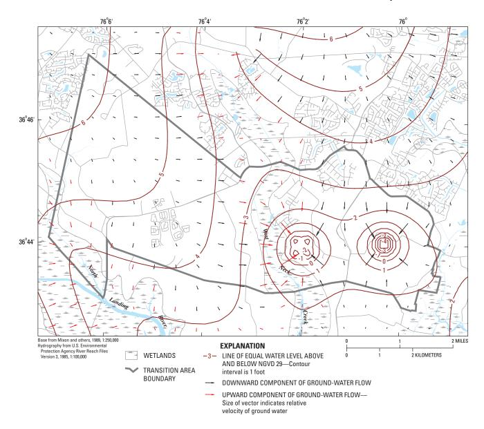
**Figure 16.** Simulated ground-water flow patterns in the sand aquifer of the Yorktown confining unit (model layer 4) caused by pumping 150,000 gallons per day at a golf course (adjacent to West Neck Creek) and 150,000 gallons per day at a hypothetical neighborhood in the Transition Area of Virginia Beach, Va.
