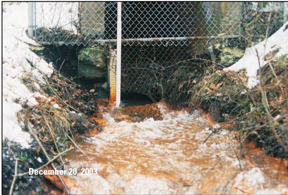
Figure 5. Mine drainage discharging from the Lykens Drift (LD) discharge in Bear Creek watershed, Dauphin County, Pennsylvania. Picture taken looking toward the source of the mine drainage. The survey rod near the center is intended for scale and extends 4 ft above the water surface.
