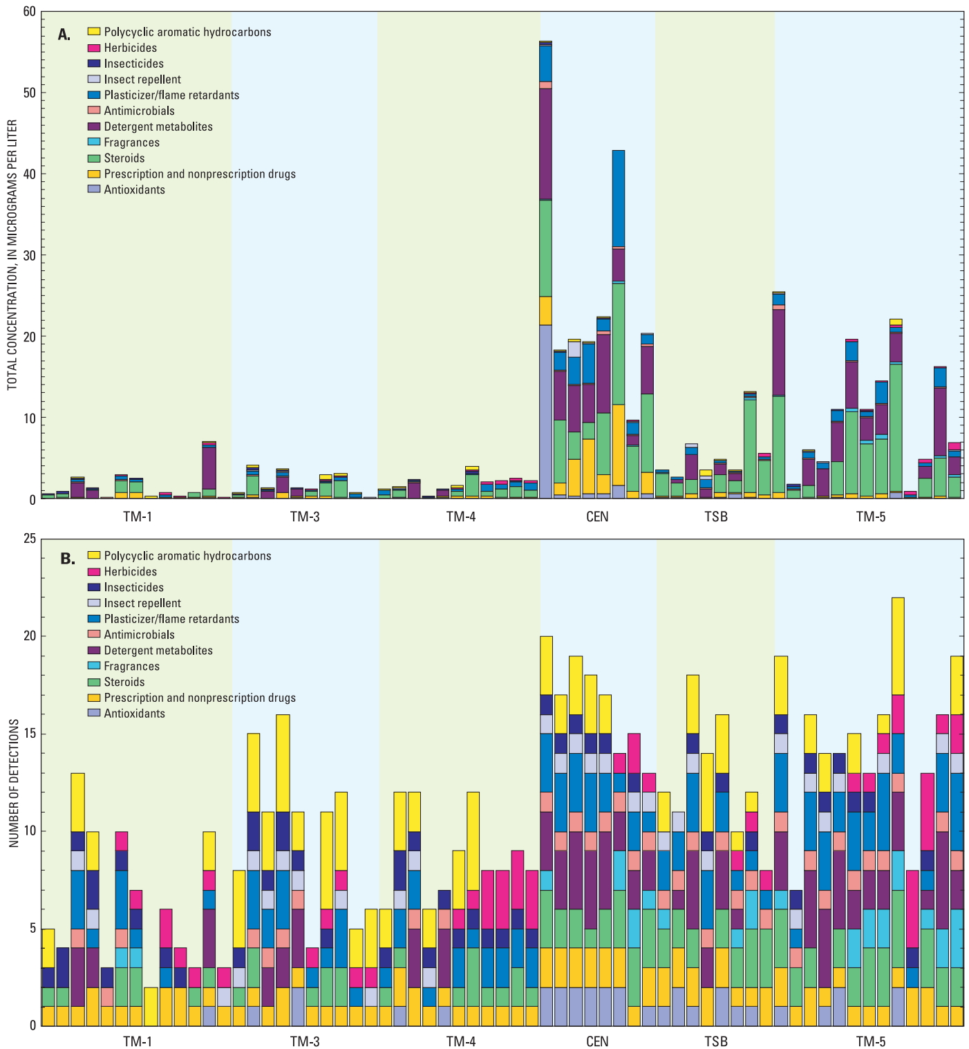
Figure 25. Summary of the types of organic wastewater compounds detected per sample for (A) total concentration (summation of 48 compounds) and (B) number of compounds detected, Threemile Creek basin, Mobile, Alabama, 2000–2003.
