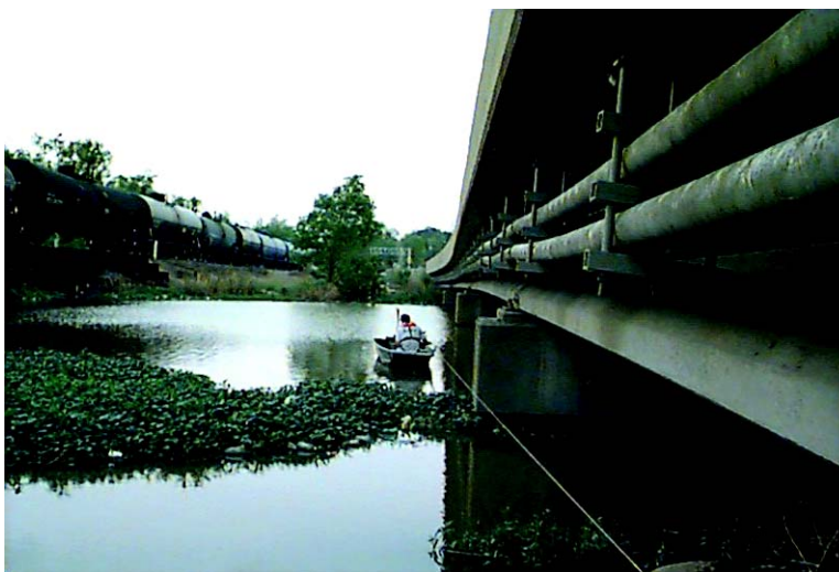
USGS personnel using an ADCP to make a discharge measurement at site TM-5 on Threemile Creek
