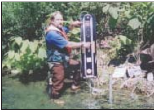
Hydrologist using a manometer board to measure head differences between surface water and ground water.
