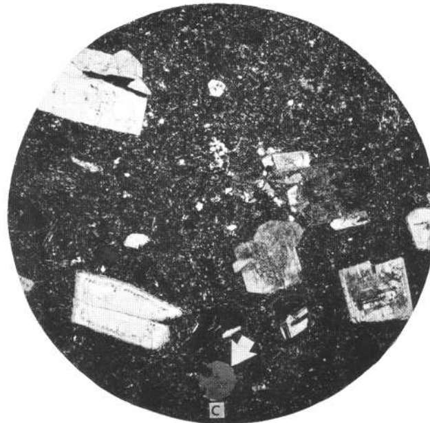
DACITE PORPHYRY: A CLOSER LOOK at two common varieties. A, Porphyry with medium-size phenocrysts of cloudy feldspar, dark biotite and hornblende, and larger egg-shaped grains of glassy quartz (white arrows). B, Porphyry with large phenocrysts of feldspar and smaller ones of biotite, hornblende, and quartz (white arrow). Natural size. C, Slice of dacite porphyry, magnified 8 times. Doubly polarized light. (Fig. 55)
