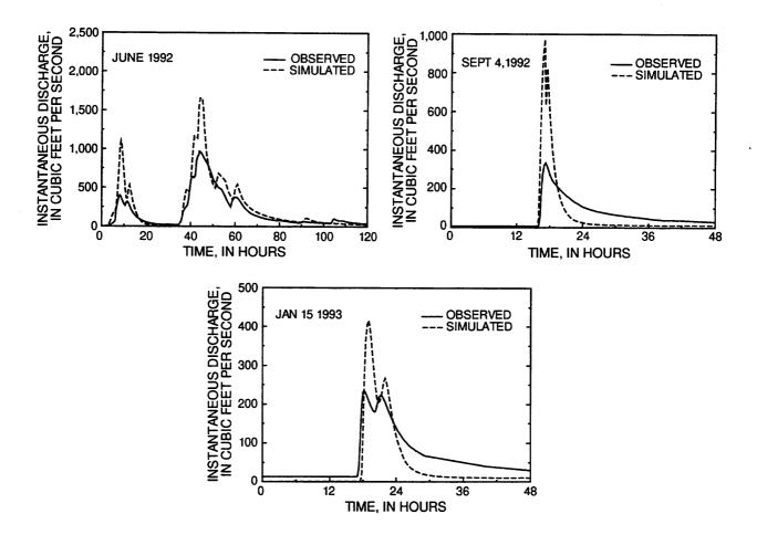
Figure 48. Typical observed hydrographs for storms occurring in the Walker Creek watershed and corresponding hydrographs simulated using the Environmental Protection Agency Storm Water Management model.
