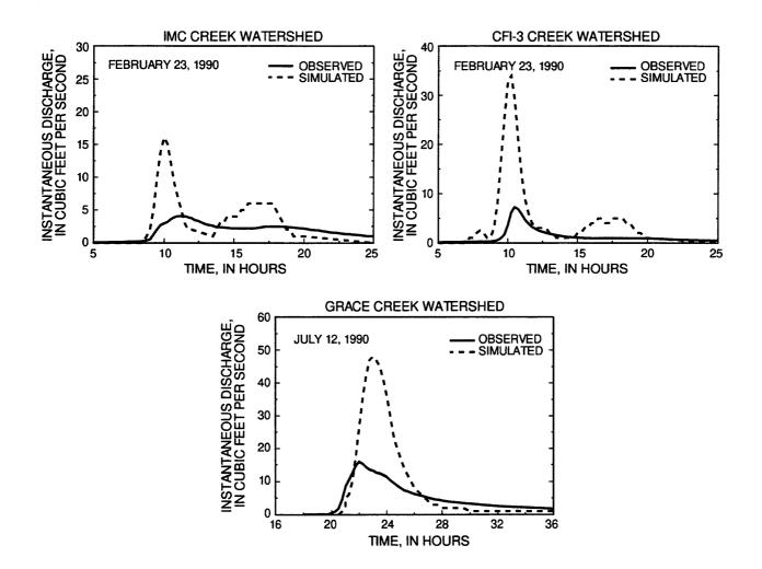
Figure 38. Typical observed hydrographs for storms occurring in the IMC, CFI-3, and Grace Creek watersheds and corresponding hydrographs simulated using the U.S. Army Corps of Engineers HEC-1 model.
