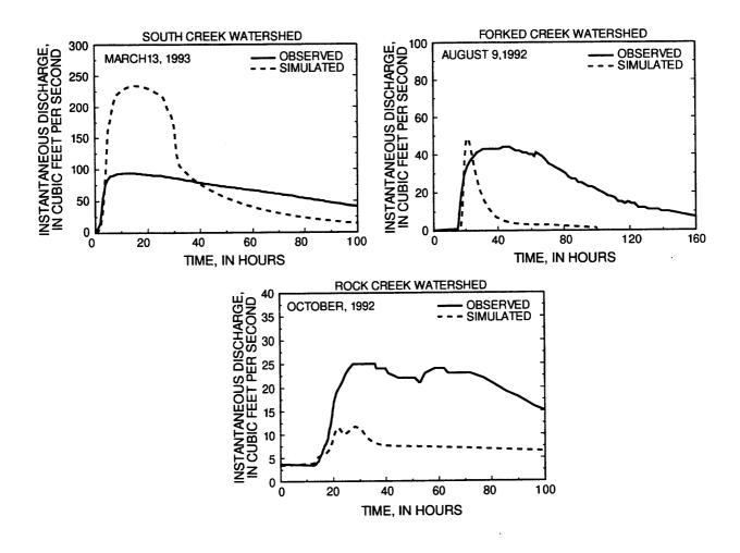
Figure 31. Typical observed hydrographs for storms occurring in the South, Forked, and Rock Creek watersheds and corresponding hydrographs simulated using the NRCS TR-20 model.
