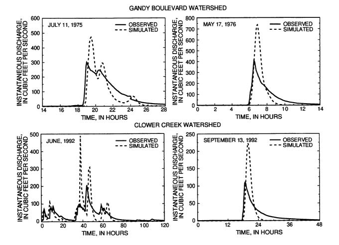
Figure 34. Typical observed hydrographs for storms occurring in the Gandy Boulevard and Clower Creek watersheds and corresponding hydrographs simulated using the U.S. Army Corps of Engineers HEC-1 model.
