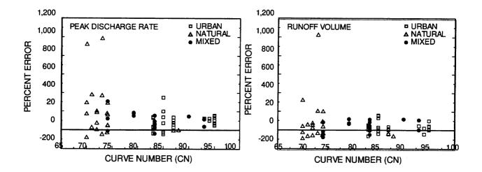
Figure 33. Comparison of the percent error between observed and estimated peak discharge rates and runoff volumes with the average curve number using the U.S. Army Corps of Engineers HEC-1 model.
