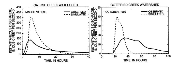
Figure 37. Typical observed hydrographs for storms occurring in the Catfish Creek and Gottfried Creek watershed and corresponding hydrographs simulated using the U.S. Army Corps of Engineers HEC-1 model.
