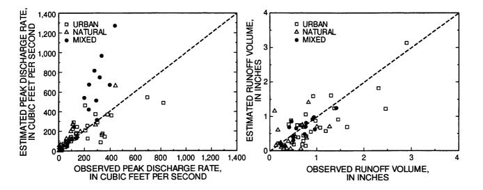
Figure 41. Comparison of observed and estimated peak discharge rates and runoff volumes for the Environmental Protection Agency Storm Water Management model, using the Horton infiltration method.
