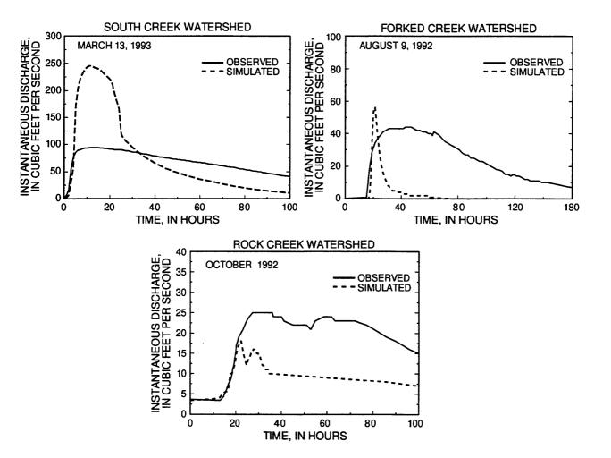
Figure 39. Typical observed hydrographs for storms occurring in the South, Forked, and Rock Creek watersheds and corresponding hydrographs simulated using the U.S. Army Corps of Engineers HEC-1 model.
