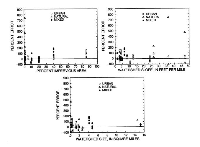
Figure 42. Comparison of the percent error between estimated and observed peak discharge rates with percent impervious area, average watershed slope, and watershed size, for the Environmental Protection Agency StormWater Management model, using Green-Ampt infiltration method.
