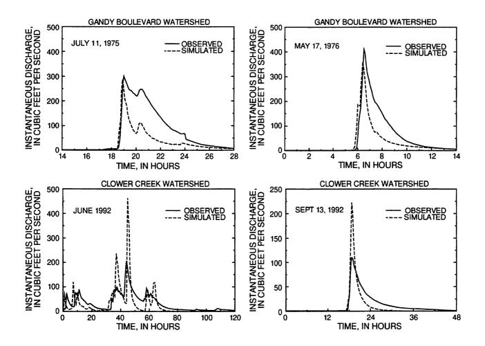
Figure 46. Typical observed hydrographs for storms occurring in the Gandy Boulevard and the Clower Creek watersheds and corresponding hydrographs simulated using the Environmental Protection Agency Storm Water Management model.
