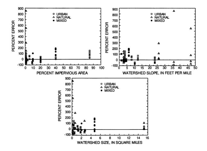
Figure 43. Comparison of the percent error between estimated and observed peak discharge rates with impervious area, average watershed slope, and watershed size, for the Environmental Protection Agency Storm Water Management model, using the Horton infiltration method.
