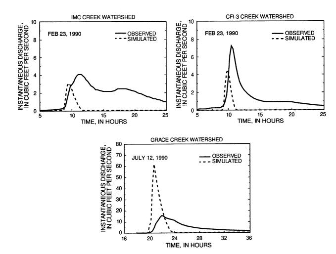
Figure 50. Typical observed hydrographs for storms occurring in the IMC, CFI-3 and Grace Creek watersheds and corresponding hydrographs simulated using the Environmental Protection Agency Storm Water Management model.
