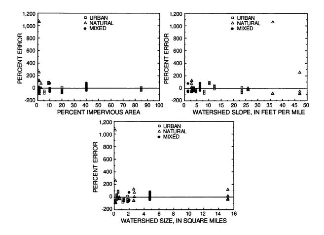
Figure 45. Comparison of the percent error between estimated and observed runoff volumes with percent impervious area average watershed slope, and watershed size, for the Environmental Protection Agency Storm Water Management model, using the Horton infiltration method.
