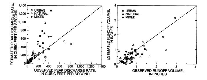
Figure 40. Comparison of observed and estimated peak discharge rates and runoff volumes for the Environmental Protection Agency Storm Water Management model, using the Green-Ampt infiltration method.
