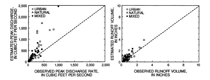
Figure 32. Comparison of the observed and estimated peak discharge rates and runoff volumes calculated using the U.S. Army Corps of Engineers HEC-1 model.
