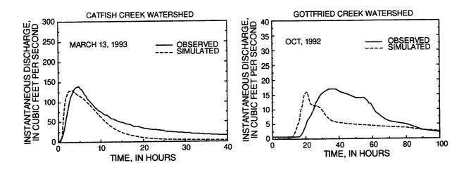
Figure 49. Typical observed hydrographs for storms occurring in the Catfish Creek and Gottfried Creek watersheds and corresponding hydrographs simulated using the Environmental Protection Agency Storm Water Management model.
