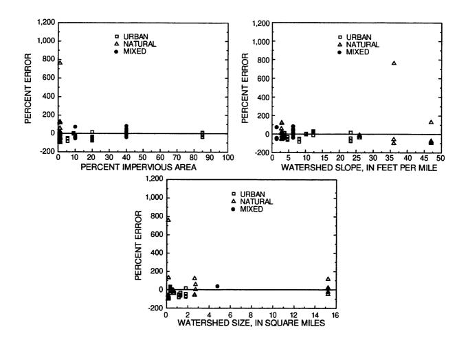
Figure 44. Comparison of the percent error between estimated and observed runoff volumes with percent impervious area, average watershed slope, and watershed size, for the Environmental Protection Agency Storm Water Management model, using the Green-Ampt infiltration method.
