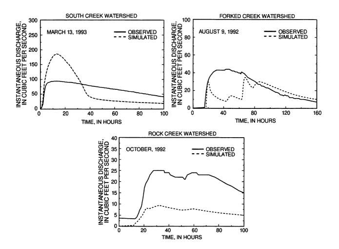
Figure 51. Typical observed hydrographs for storms occurring in the South, Forked, and Rock Creek watersheds and corresponding hydrographs simulated using the Environmental Protection Agency Storm Water Management model.
