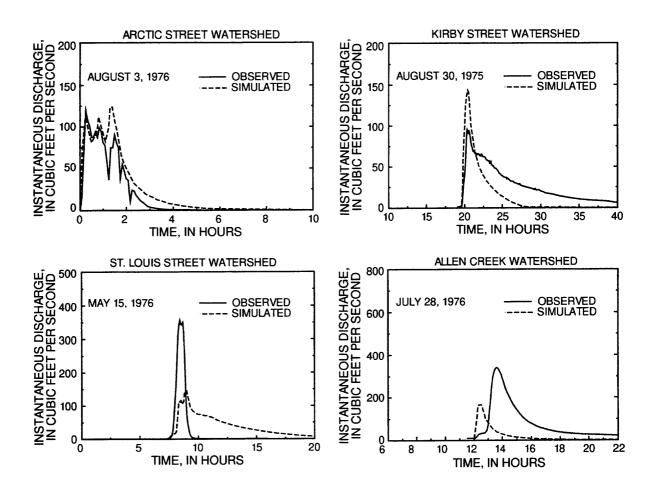
Figure 47. Typical observed hydrographs for storms occurring in the Arctic Street, Kirby Street, St. Louis Street and Aller Creek watersheds and corresponding hydrographs simulated using the Environmental Protection Agency Storm Water Management model.
