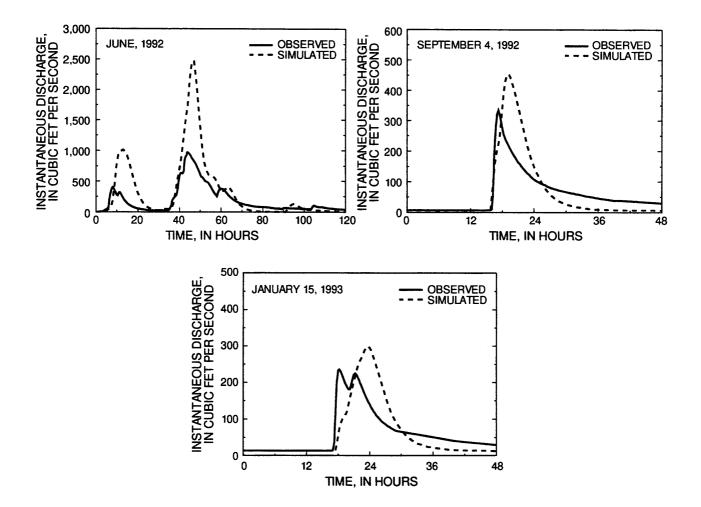
Figure 36. Typical observed hydrographs for storms occurring in the Walker Creek watershed and corresponding hydrographs simulated using the U.S. Army Corps of Engineers HEC-1 model.
