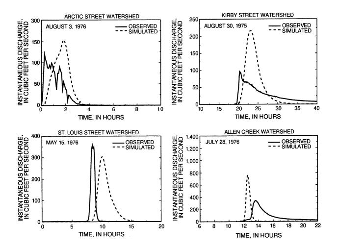
**Figure 35**. Typical observed hydrographs for storms occurring in the Arctic Street, Kirby Street, St. Louis Street, and Allen Creek watersheds and corresponding hydrographs simulated using the U.S. Army Corps of Engineers HEC-1 model.
