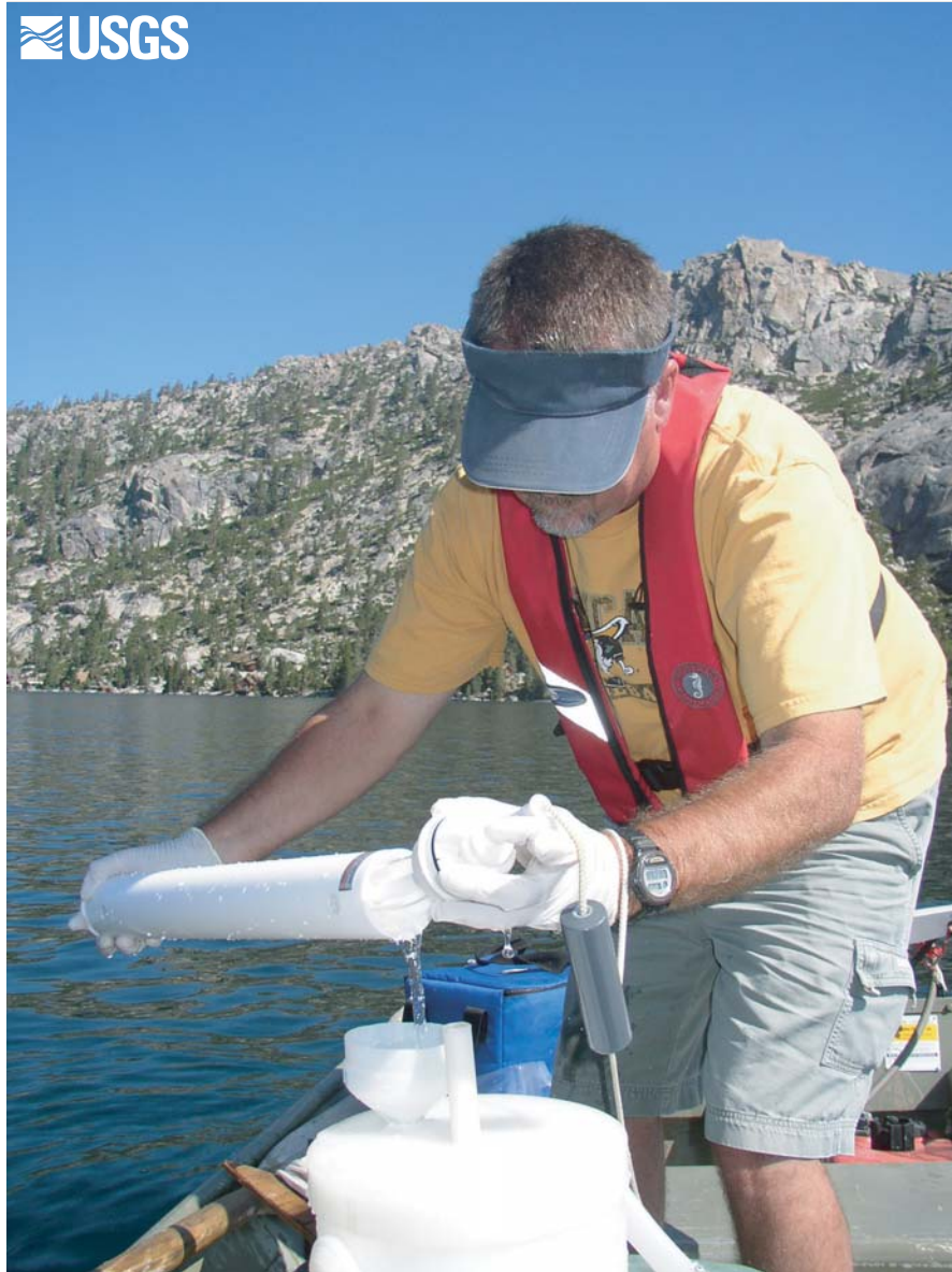
Figure 4. Sample collection at Lower Echo Lake. An all-Teflon sampler was used to obtain samples from various depths in the lakes.
