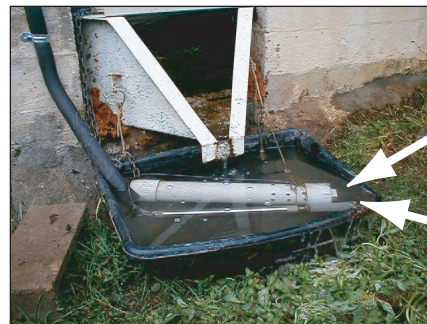
Figure 3. Water-quality monitoring and volatile organic compound sampling equipment at Wilson Spring.
