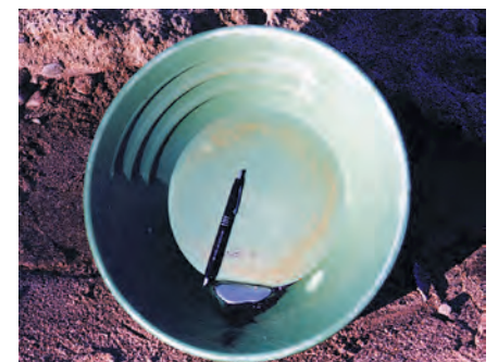
Figure 3. Gold pan with more than 30 grams of mercury from 1 kilogram of mercury-contaminated sediments collected in a drainage tunnel.
