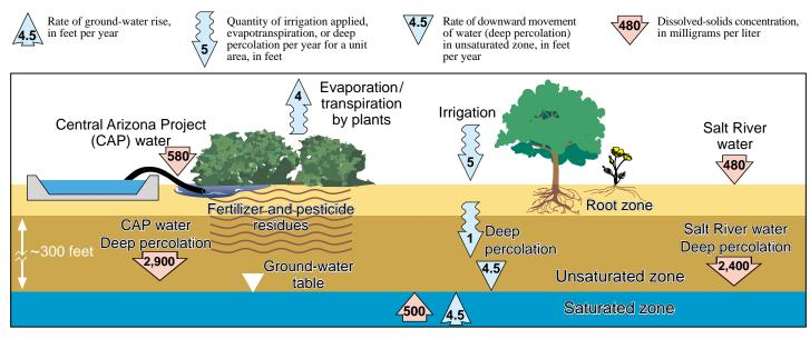
Diagrammatic illustration showing quantity of irrigation, evapotranspiration, or deep percolation; rate of ground-water movement; and dissolved-solids concentration for waters in the Salt River Valley, Phoenix, Arizona.
