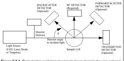
**Figure 6.7-1.** Photoelectric nephelometer (single-beam design) showing optional additional detectors for ratiometric, backscatter, or transmitted determination of turbidity. [Modified from Sadar (1998)].
