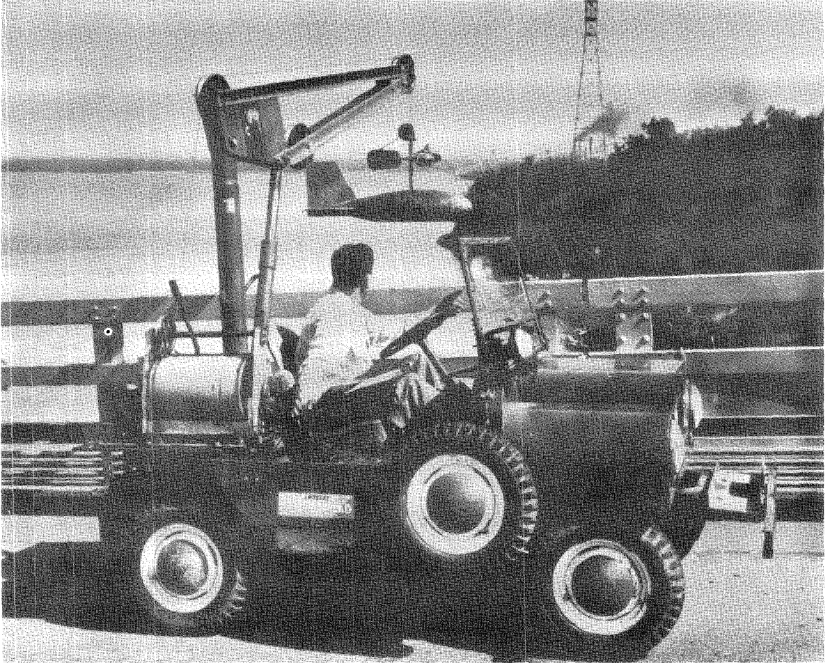
Figure 44.—Truck-mounted crane used on the Mississippi River.
