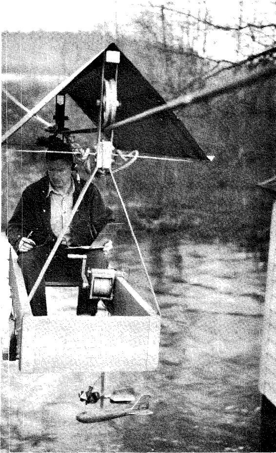
Figure 40.—Sitdown cable car with Canfield reel clamped to side of car.
