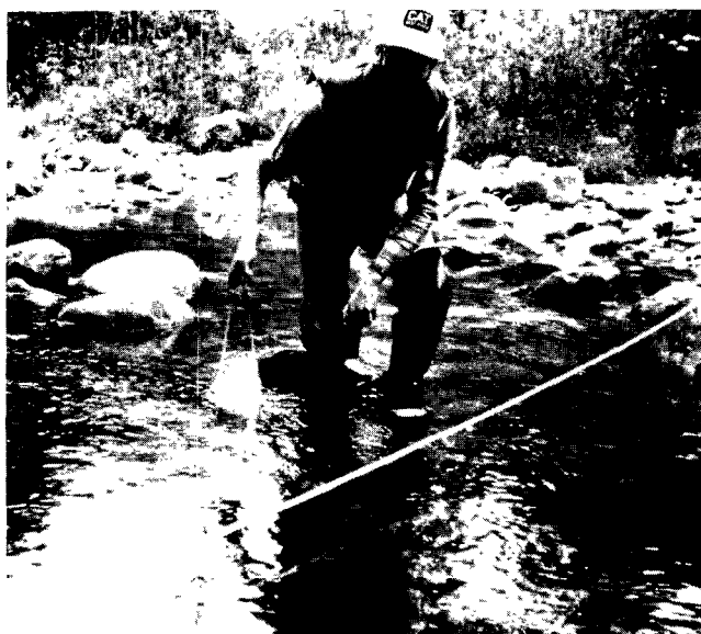
Figure 19.—Collecting gas sample at selected point in measuring section.
