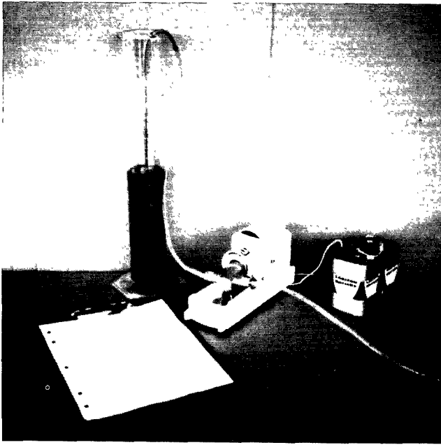
Figure 13.—Pump and graduated cylinder used for constant-rate dye injection.
