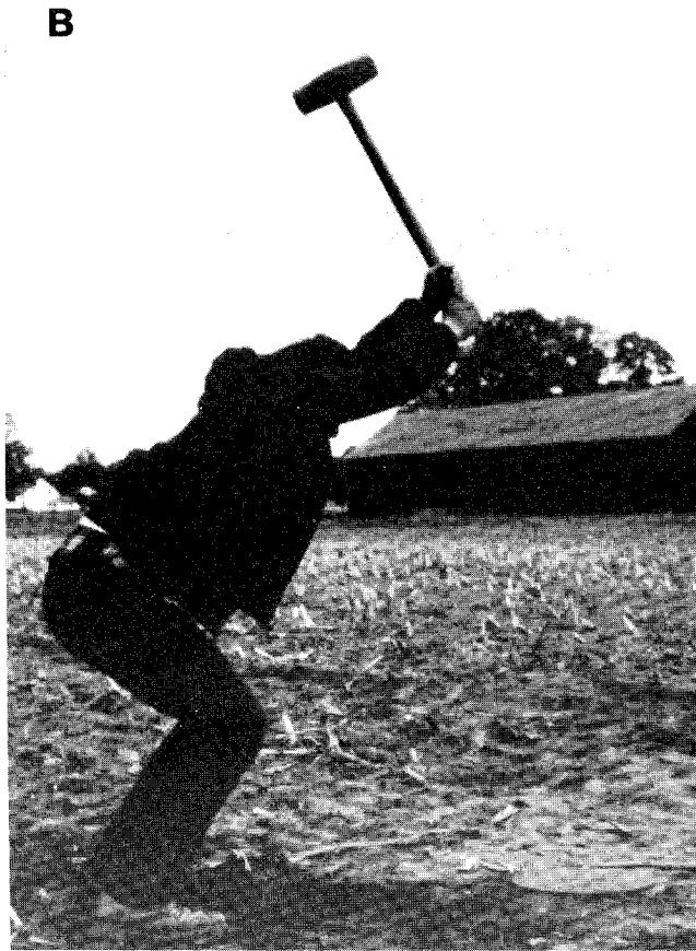
Figure 32.—Commonly used seismic energy sources: A, Shotgun; B, Sledge hammer; C, Explosives; D, Weight drop.
