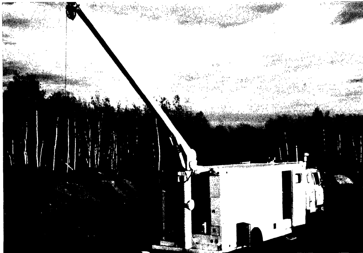
Figure 22.—Large logging truck used for deep-well logging.
