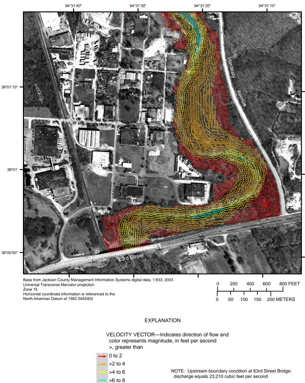
Downstream boundary condition at lower Blue Parkway Bridge: stage elevation equals 756 feet
