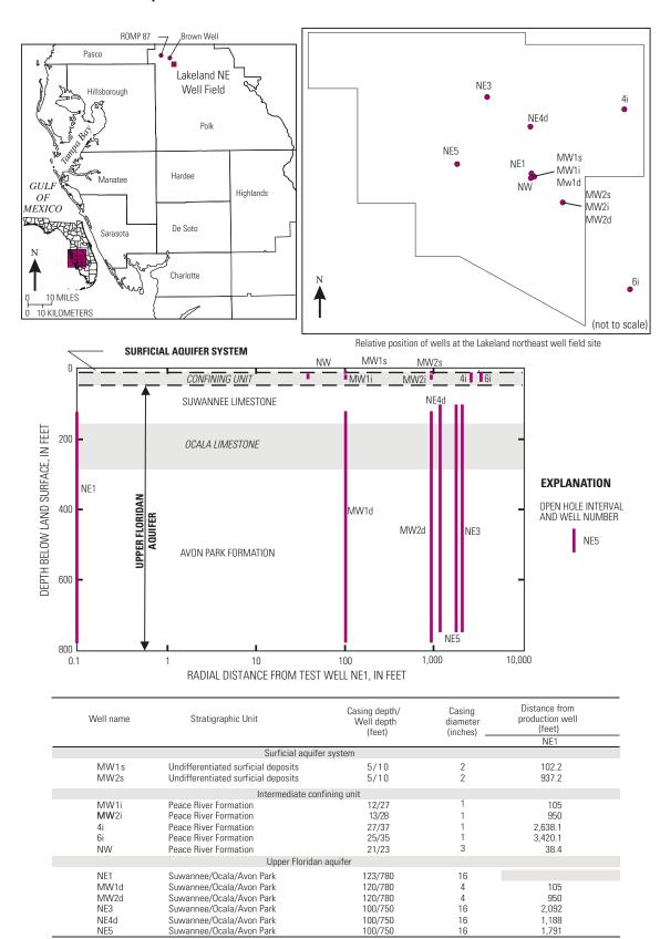
**Figure 45**. Generalized hydrogeologic section and location, plan view, description and configuration of wells at the Lakeland Northeast Well Field test site.
