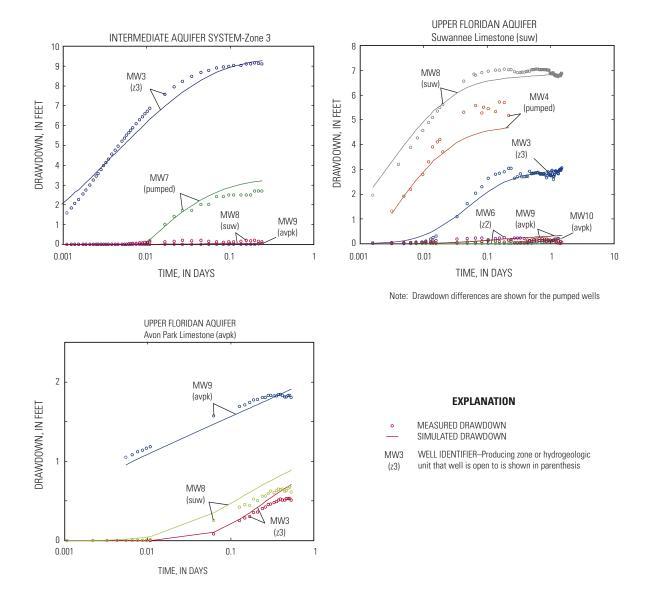
Figure 28. Simulated and measured drawdown for the three aquifer tests conducted at the ROMP 22 test site.
