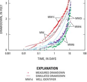
**Figure 47.** Simulated and measured drawdown for the Upper Floridan aquifer test conducted at the Lakeland Northeast Well Field test site.
