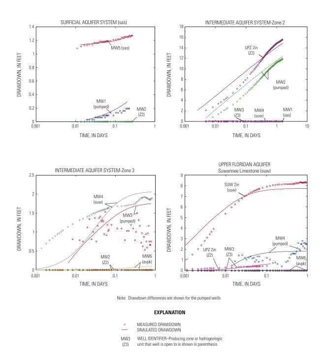
Figure 8. Simulated and measured drawdown for the four aquifer tests conducted at the ROMP 5 test site.
