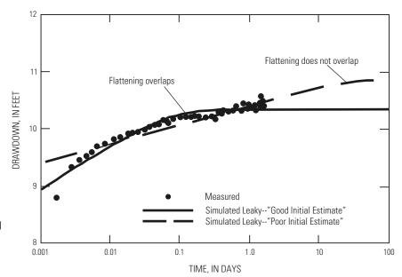
**Figure 4.** Effect of poor initial parameter estimates on model fit.
