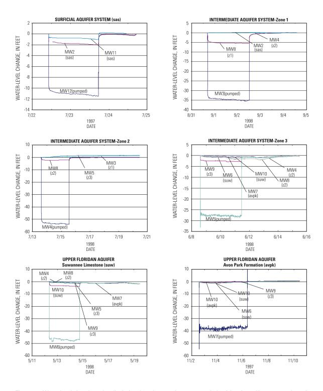
**Figure 14.** Water levels in selected wells during drawdown and recovery periods of the six aquifer tests conducted at the ROMP 12 test site.
