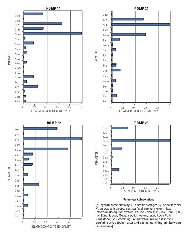
Figure 22. Relative composite sensitivity for final parameter values for ROMP 14, 20, 22, and 25.
