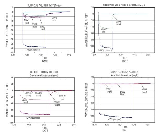
**Figure 20.** Water levels in selected wells during drawdown and recovery periods of the four aquifer tests conducted at the ROMP 14 test site.
