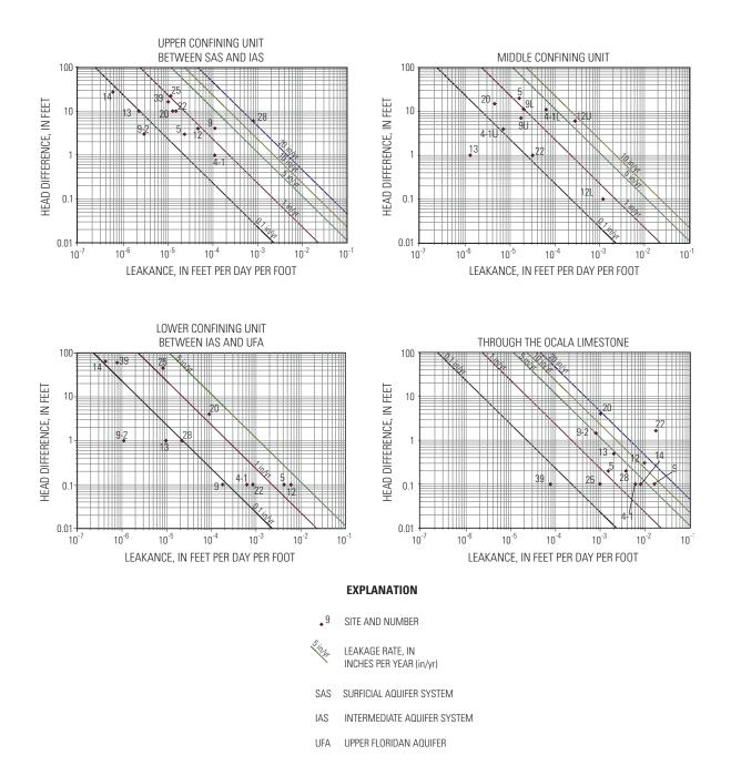
Figure 49. Comparison between simulated leakance values, head differences, and leakage rates across confining units at selected sites.
