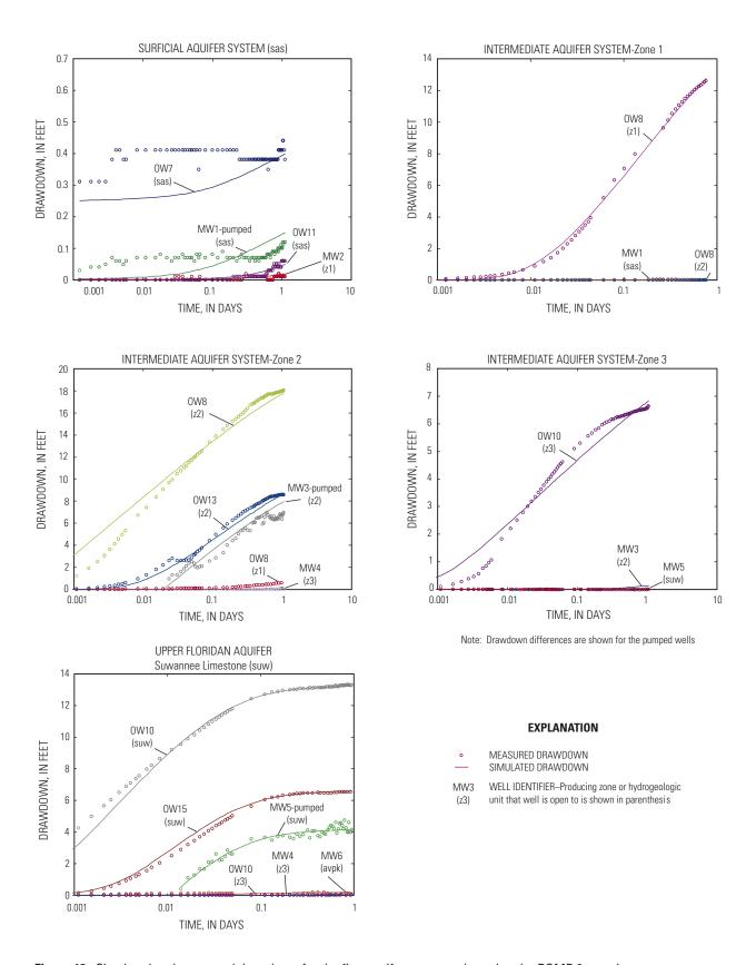
Figure 12. Simulated and measured drawdown for the five aquifer tests conducted at the ROMP 9 test site.
