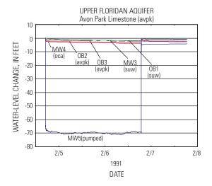
**Figure 43.** Water levels in selected wells during drawdown and recovery periods of the Avon Park aguifer test conducted at the ROMP TR 9-2 test site.
