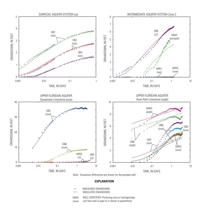
Figure 34. Simulated and measured drawdown for the four aquifer tests conducted at the ROMP 28 test site.
