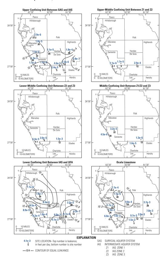
**Figure 48.** Distribution of leakance values estimated from numerical analyses of aquifer-test data collected at test sites.
