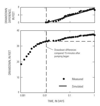
**Figure 5.** Effects of simulating drawdown in production wells after entry losses have stablized.
