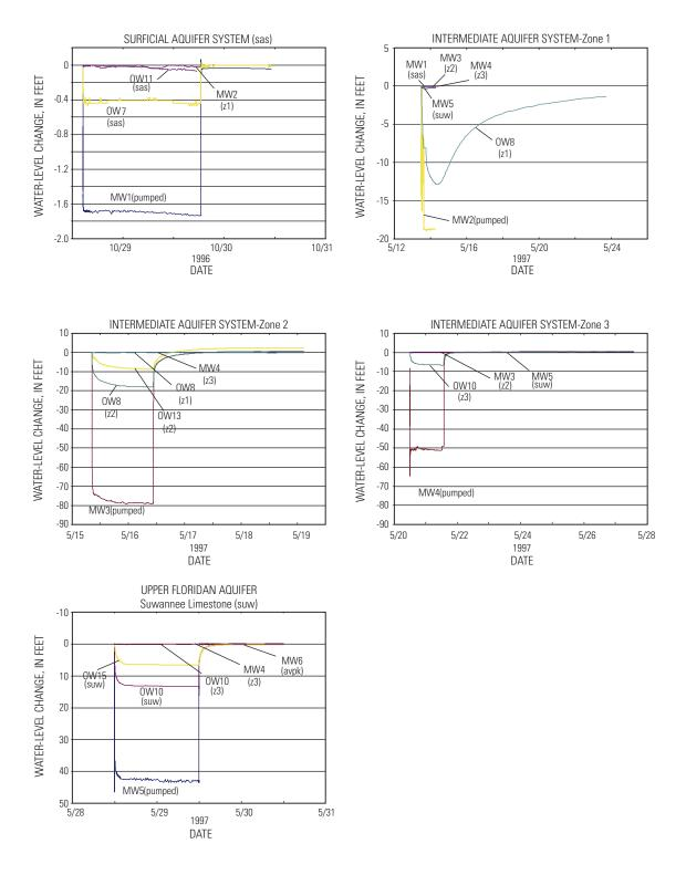
**Figure 11.** Water levels in selected wells during drawdown and recovery periods of the five aquifer tests conducted at the ROMP 9 test site.
