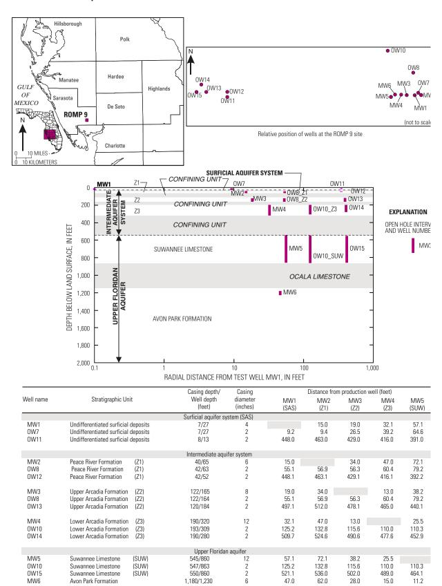
Figure 10. Generalized hydrogeologic section and location, plan view, description and configuration of wells at the ROMP 9 test site.
