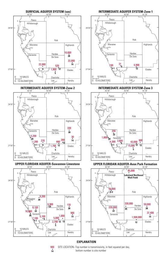
**Figure 50.** Transmissivity of the pumped zones based on aquifer thickness and simulated horizontal hydraulic conductivity from numerical models.
