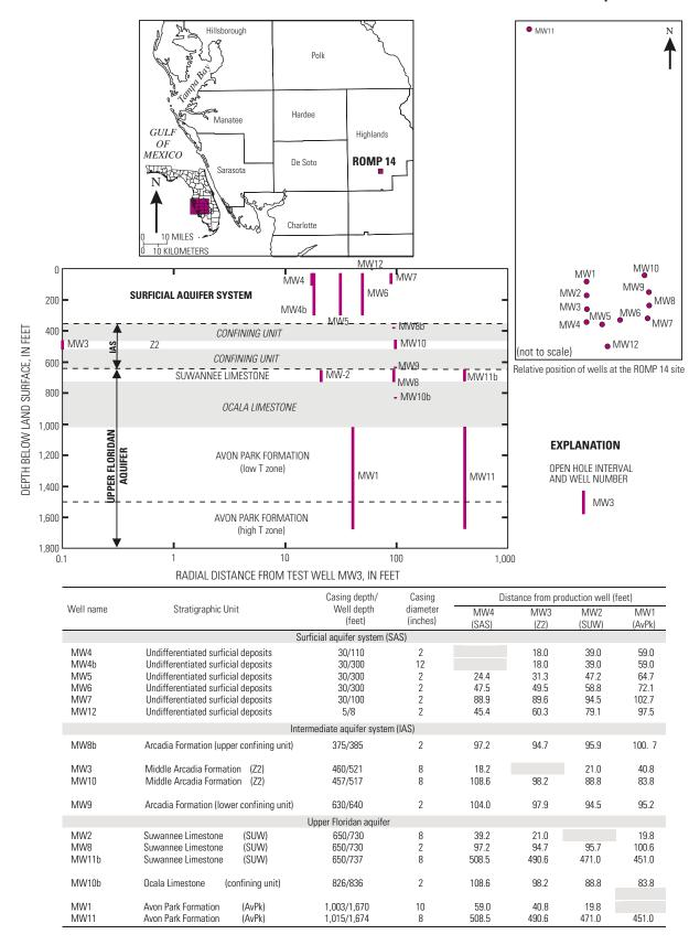
Figure 19. Generalized hydrogeologic section and location, plan view, description and configuration of wells at the ROMP 14 test site.
