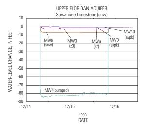
Figure 27. Water levels in selected wells during drawdown and recovery periods of the three aquifer tests conducted at the ROMP 22 test site.
