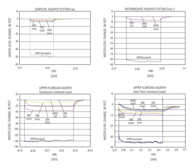
Figure 33. Water levels in selected wells during drawdown and recovery periods of the four aquifer tests conducted at the ROMP 28 test site.
