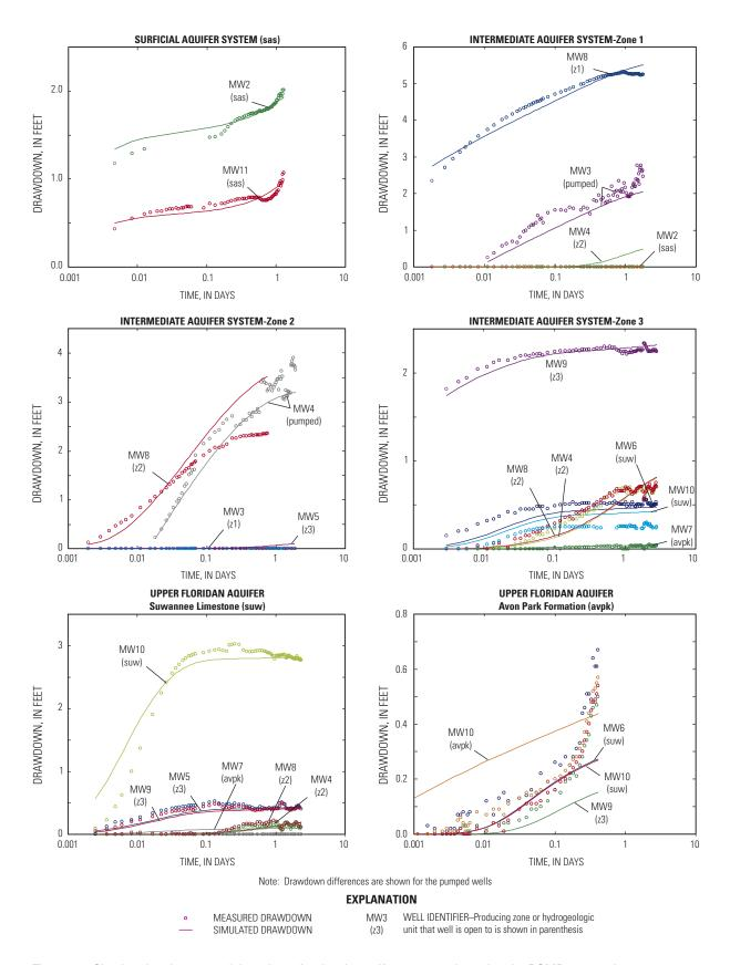
Figure 15. Simulated and measured drawdown for the six aquifer tests conducted at the ROMP 12 test site.
