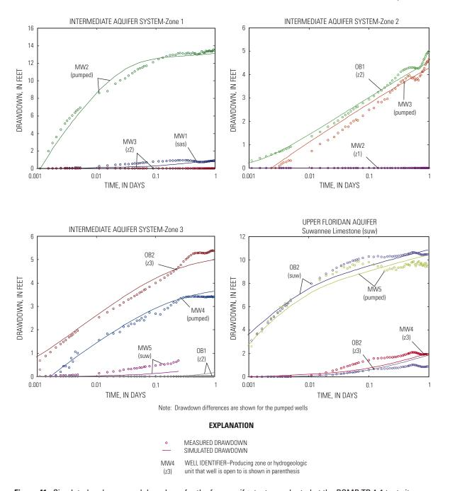
Figure 41. Simulated and measured drawdown for the four aquifer tests conducted at the ROMP TR 4-1 test site.
