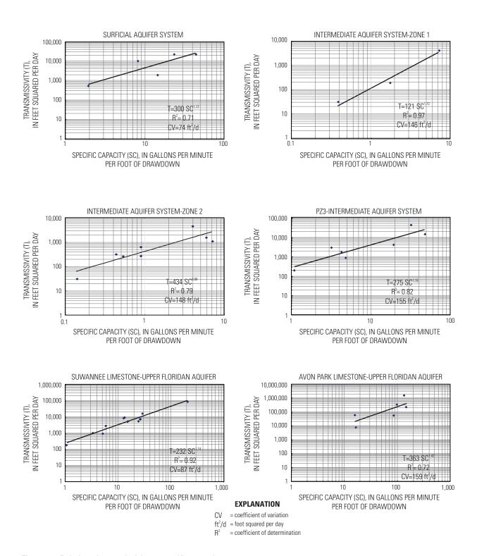
Figure 51. Relation of transmissivity to specific capacity.
