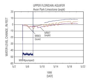
Figure 30. Water levels in selected wells during drawdown and recovery periods of the two aquifer tests conducted at the ROMP 25 test site.
