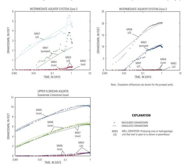
Figure 25. Simulated and measured drawdown for the three aquifer tests conducted at the ROMP 20 test site.
