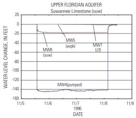
**Figure 17.** Water levels in selected wells during drawdown and recovery periods of the three aquifer tests conducted at the ROMP 13 test site.
