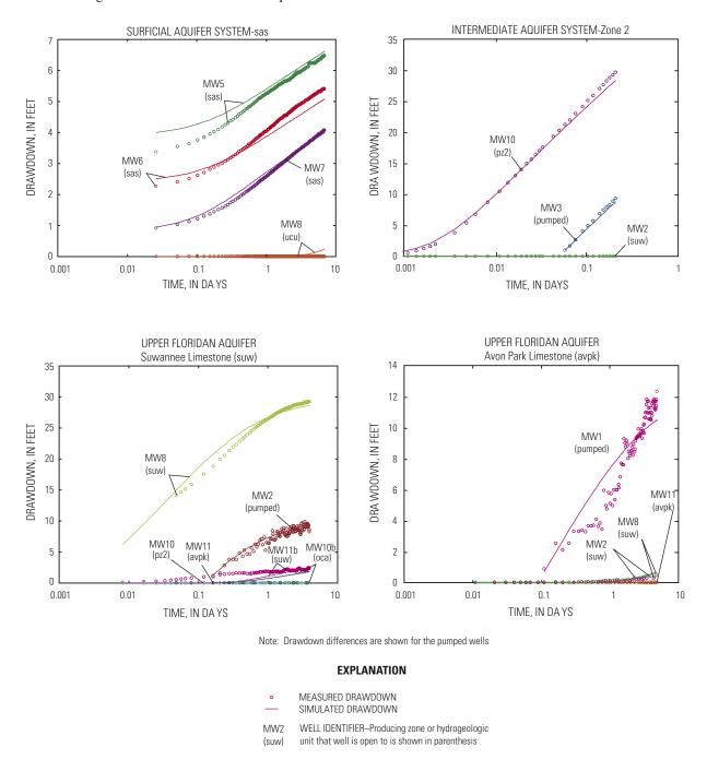
Figure 21. Simulated and measured drawdown for the four aquifer tests conducted at the ROMP 14 test site.
