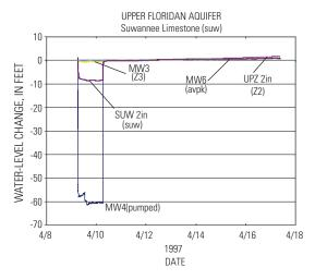
Figure 7. Water levels in selected wells during drawdown and recovery periods of the four aquifer tests conducted at the ROMP 5 test site.
