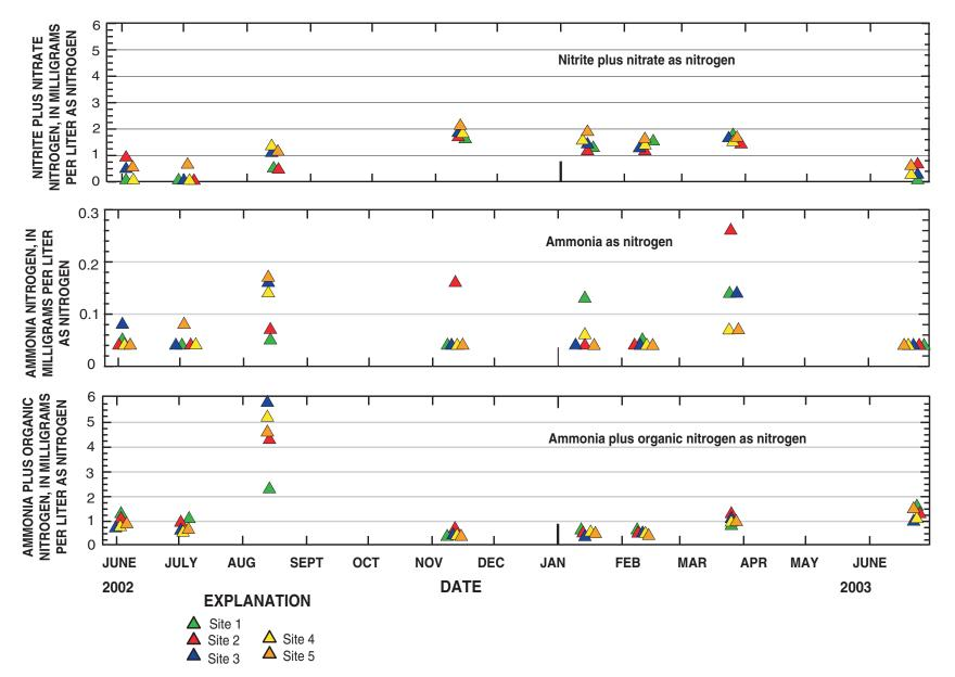
Figure 5. Distribution of nitrite plus nitrate as nitrogen, ammonia as nitrogen, ammonia plus organic nitrogen as nitrogen concentrations measured in surface-water quality samples from sites 1-5 on Turkey Creek, northwest Oklahoma, June 2002 to June 2003.
