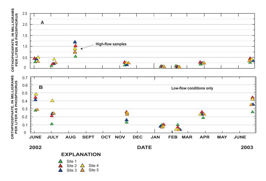
**Figure 7.** Distribution of concentrations of orthophosphate in surface-water quality samples from sites 1-5 on Turkey Creek, northwest Oklahoma, June 2002 to June 2003. Plot A shows concentrations of all samples, plot B shows concentrations of samples collected during low-flow conditions only.
