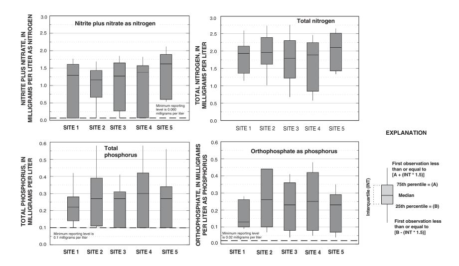
**Figure 4.** Distribution of nutrient concentrations measured in surface-water quality samples during low-flow conditions at sites 1-5 on Turkey Creek, northwest Oklahoma, June 2002 to June 2003. Each box plot was constructed from seven analyses.
