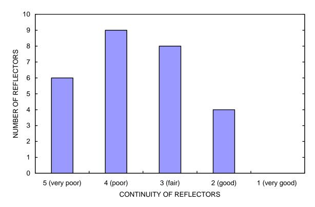
Figure 13. Distribution of interpreted borehole-radar reflectors sorted by the continuity of the reflectors, Project Shoal Area, Churchill County, Nevada.
