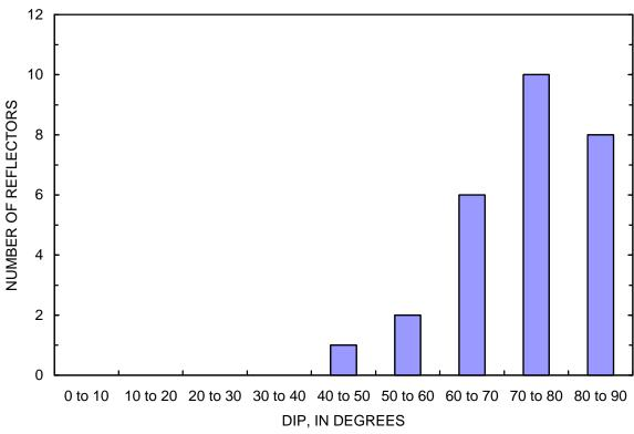
**Figure 12.** Distribution of interpreted borehole-radar reflectors sorted by dip, Project Shoal Area, Churchill County, Nevada.
