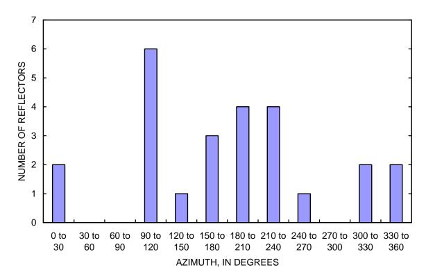
Figure 11. Distribution of interpreted borehole-radar reflectors sorted by azimuth, Project Shoal Area, Churchill County, Nevada.
