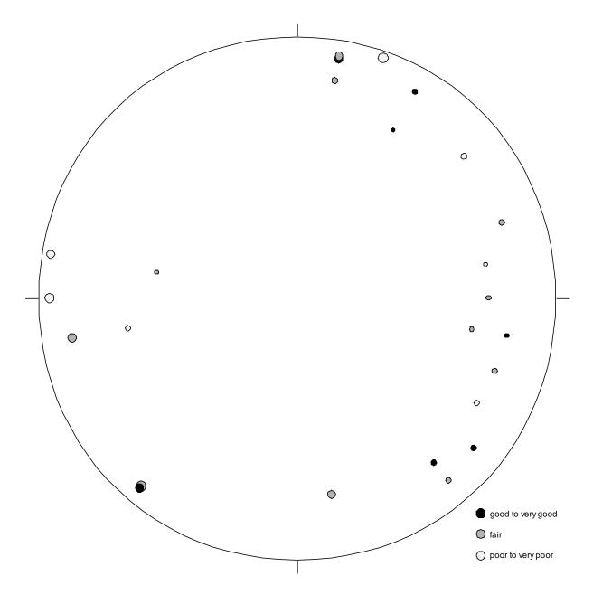
Figure 15. Lower hemisphere equal-area stereo-net showing poles of all interpreted radar reflectors, weighted by reflector length and combined reflector quality, Project Shoal Area, Churchill County, Nevada.
