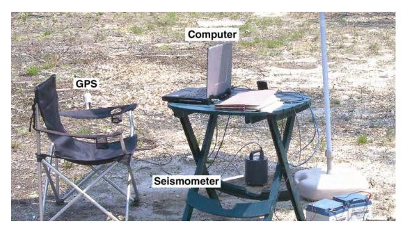
Figure 4: Three-component seismometer connected to field laptop for H/V seismic surveys.
