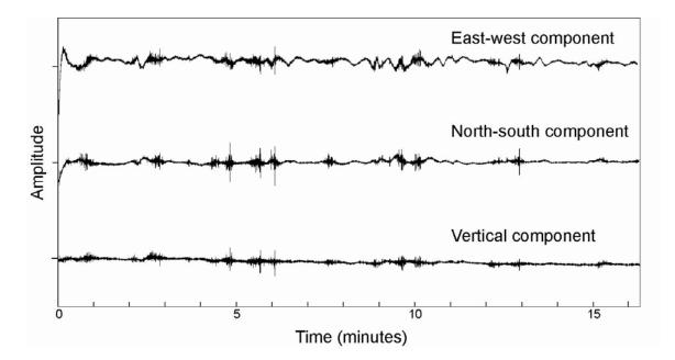
**Figure 5:** Representative 3-component ambient noise seismic records from Truro, Cape Cod, Massachusetts.
