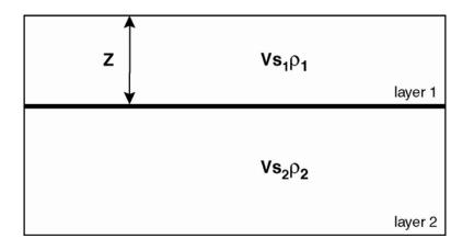
**Figure 1:** Conceptual earth model for H/V seismic method. The method assumes  $Vs_2\rho_2 \ge 2Vs_1\rho_1$ , where  $Vs_1$  and  $Vs_2$  are the shear wave velocities in layers 1 and 2, respectively, and  $\rho_1$  and  $\rho_2$  are the densities in layers 1 and 2, respectively. Z is the thickness of layer 1 (sediment).
