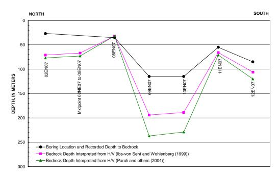
**Figure 9:** Profile of bedrock surface along transect near Firth, Nebraska, interpreted from H/V results, and depth to rock from adjacent boring logs.
