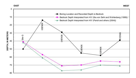
**Figure 10:** Profile of bedrock surface along transect near Oakland, Nebraska, interpreted from H/V results, and depth to rock from adjacent boring logs.
