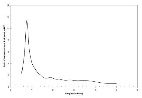
**Figure 6:** H/V spectral plot of ambient-noise seismic data from First Encounter Beach, Cape Cod, Massachusetts.
