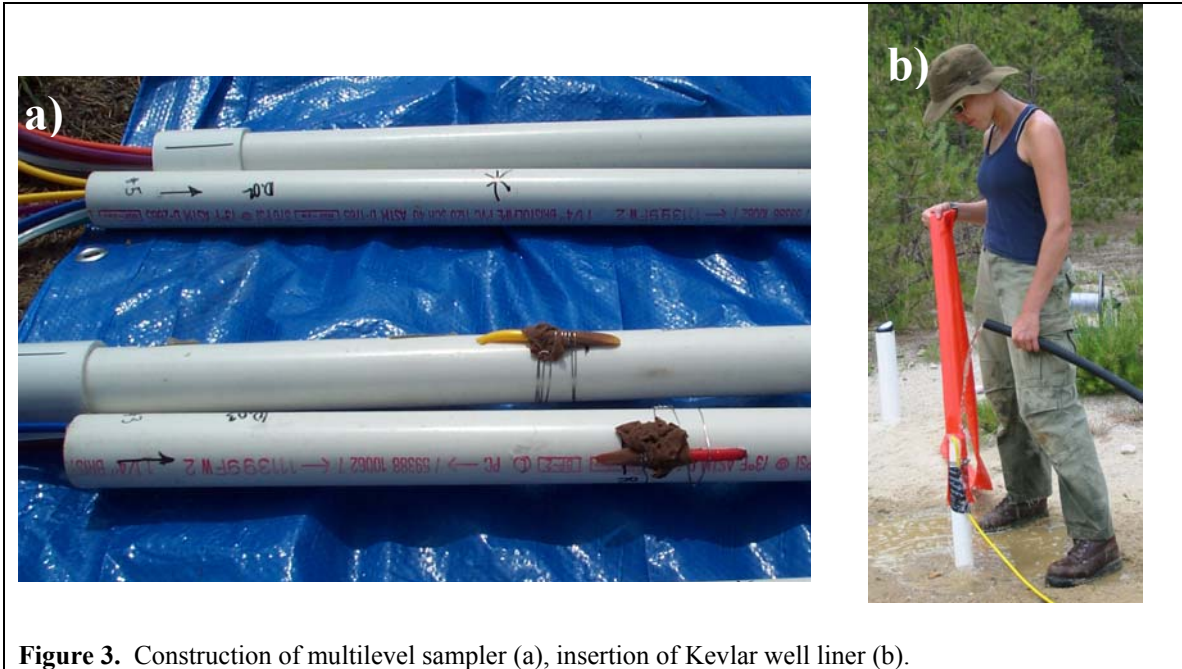
Figure 3. Construction of multilevel sampler (a), insertion of Kevlar well liner (b).
