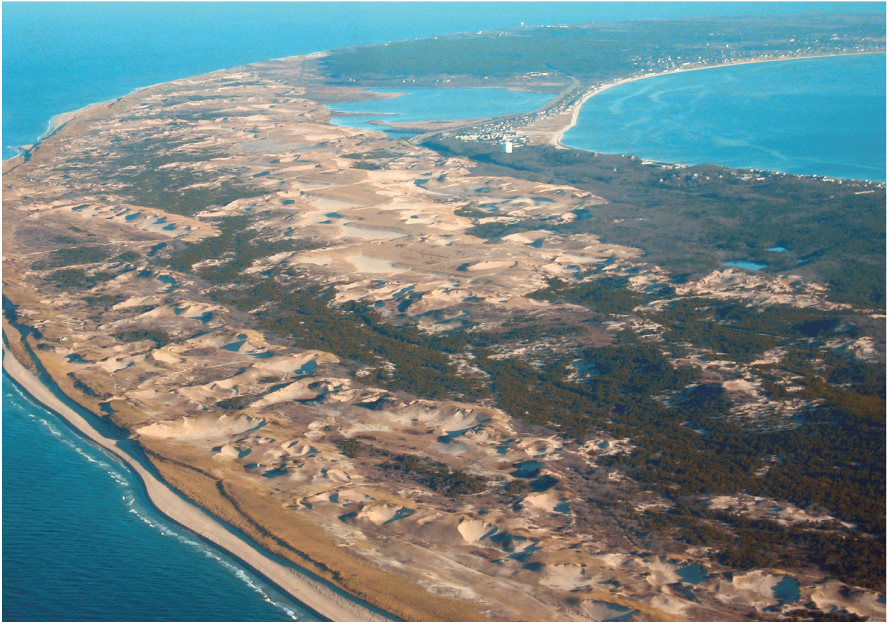
Figure 2. The Pilgrim flow lens, like the other flow lenses of the Lower Cape Cod aquifer system, is bounded laterally by the Atlantic Ocean and Cape Cod Bay. Rainfall that reaches the water table as recharge eventually leaves the aquifer system as ground-water discharge along the coast. View looking southeast.
